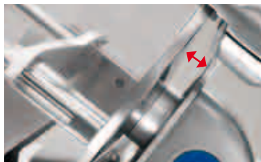
Increased gap between blade and machine body
